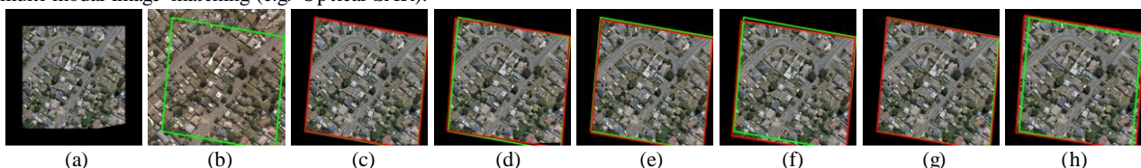
Figure 6. Registration Result of an image pair in Optical-Optical dataset. (a) Randomly affine transformed and cropped sensed image. (b) Reference image. (c) MU-Net. (d) SIFT. (e) RIFT. (f) CFOG. (g) DLKFM. (h) DLIR. The green line represents the ground truth registration result, and the red line represents the experimental registration result for each method.
