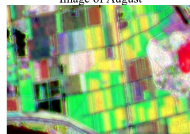
D-value of NDVI by the image of June, August and October Figure 7. The phenological feature is more prominent in the differences between grain crops and artificial turf (green: early season rice, yellow: artificial turf)
