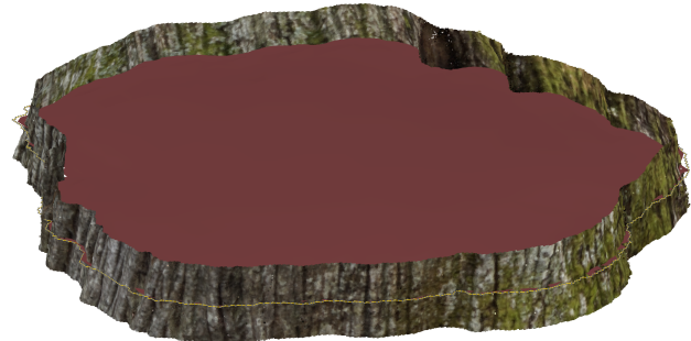
Figure 1. Mesh of the DBH section from the RGB reflex point cloud. The red color represents the surface created by the section contour (yellow line).
