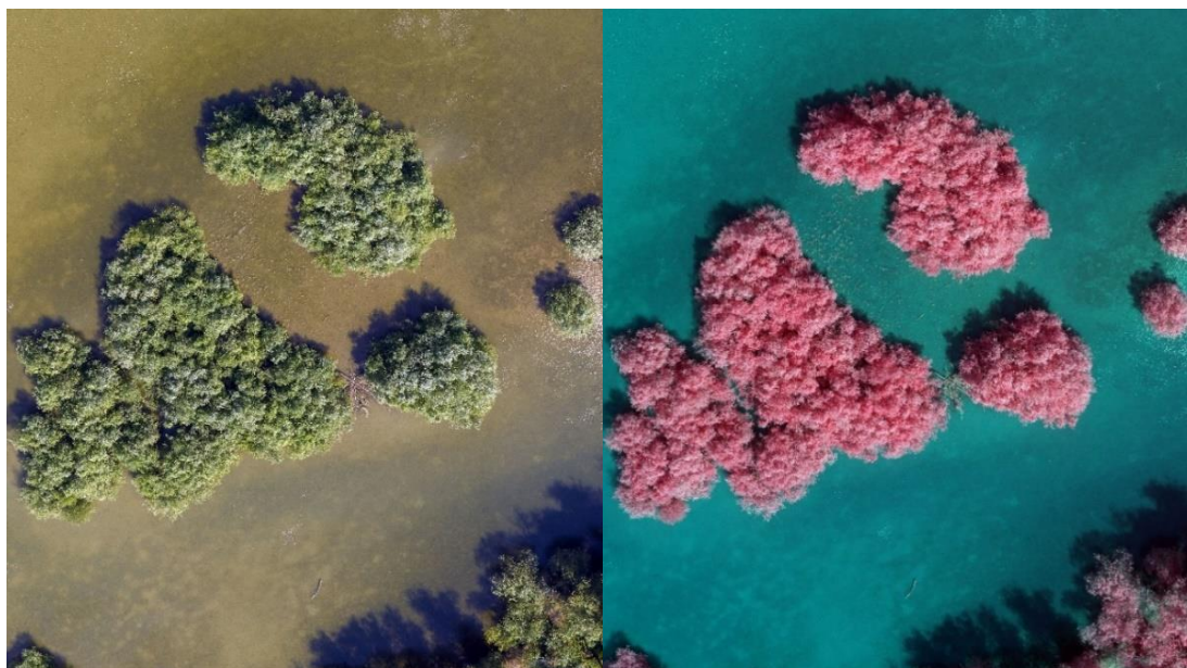
Figure 2. True Color Image of flooded area (left) and false-color composite (right) revealing chlorophyll
