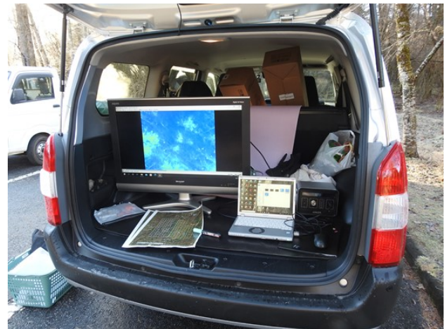
Figure 5. A mobile identification station to identify sika deer in the video acquired by a drone. It consists of a mobile power generator, a laptop pc connected to a 32-inch monitor and a printed map of the grided flight area.
