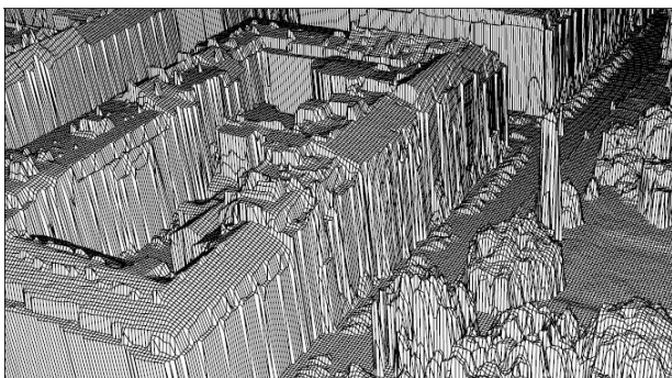
Figure 5. Using LiDAR to reconstruct a terrain model in Vienna (Rottensteiner & Briese, 2002)
