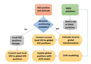
Figure 2. Flowchart for the sensor fusion approach
