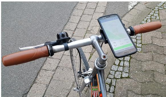
Figure 1. Measurement setup: smartphone with a solid holder attached to a bicycle's handlebar.
