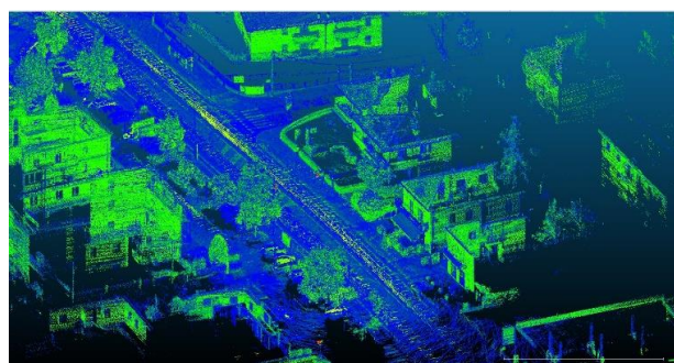
Figure 9. 3D point cloud by Kaarta Stencil 2 obtained surveying Via San Polo
