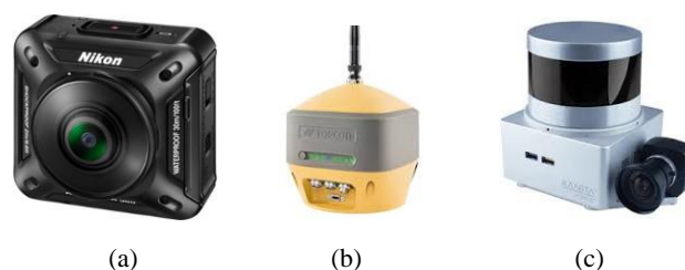
Figure 3. The instruments used in this survey. (a) Camera Nikon Key Mission 360. (b) Hiper Hr receiver by Topcon. (c) Laser Scanner Kaarta Stencil 2.
