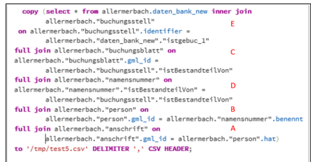
Figure 9: SQL code for automatic relational connection between the tables according to the specified relation types.
