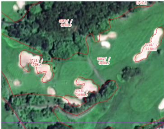
Figure 7. referring to Digital Orthophoto Image, the sandy surface is incorrectly collected as a structure
