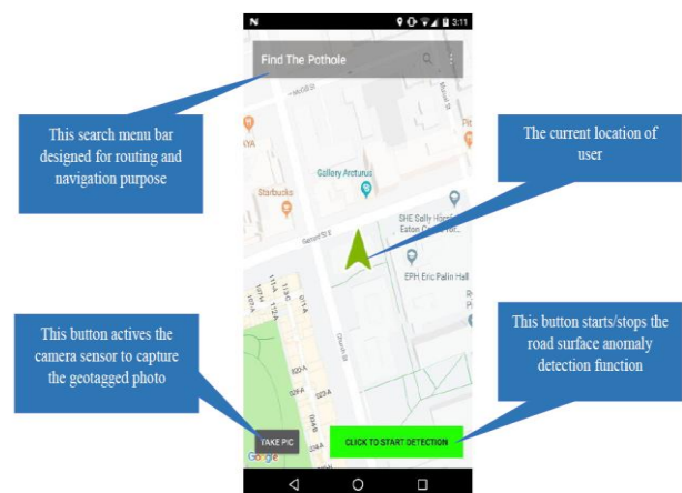
Figure 3. The main interface of the developed Mobile GIS application and its functionalities
