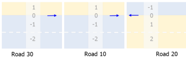
Figure 2. Lane linkage in OpenDRIVE standard (ASAM e.V., 2022)
