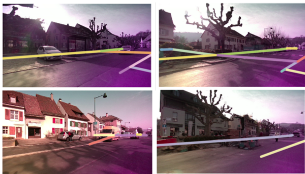
Figure 3. Examples of street centre line cues that are difficult to read because of a complex network situations (top), because of registration error (bottom left) or lack of directional information (bottom right) (images: (Nebiker et al., 2021); geo-data: (Bundesamt für Landestopografie swisstopo, 2021)).
