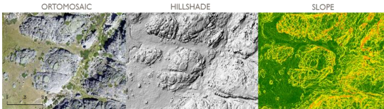
Figure 3. Models used to support the geosite analysis: orthomosaic, shadow and slope. Example from the Covão do Boi geosite.
