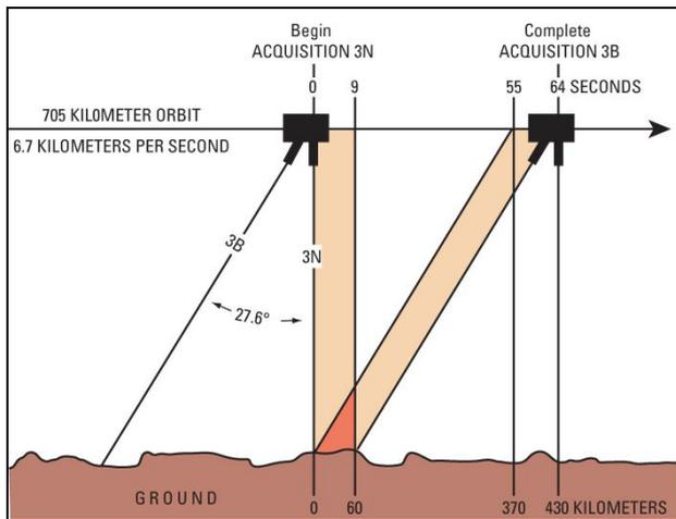
**Figure 1.** Viewing geometry for ASTER stereo data acquisition. Nadir- and backward-looking telescopes image the same area, 64 seconds apart.
