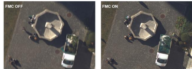
Figure 4: Leica MFC150 with FMC off/on - showing the benefit of FMC for long exposure at low sun angle (1/200 sec at 120 kn)
