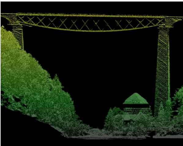
Figure 6: Profile view of a LiDAR point cloud from a Leica TerrainMapper-2, with a conical scan pattern. The result shows the enhanced details on vertical surfaces and even on the structures under the bridge deck.
