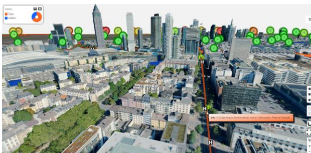
Figure 2: 3D Mesh, downtown Frankfurt, from CityMapper-2 hybrid sensor data. with transportation information
