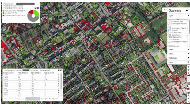
Figure 14: Hexagon M.App Enterprise to derive and visualize changes in impervious areas based on hybrid sensor data and GeoAI analysis.
