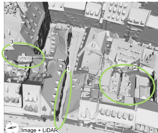
Figure 12: Comparison of 3D Mesh from image only (top) and image + LiDAR (below) approach. 3D mesh generated by Melown technologies from CityMapper-2 data, 5 cm GSD
