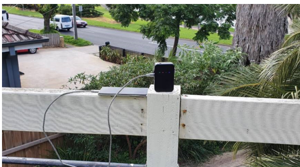
Figure 2. The Softbank GNSS QZSS enabled receiver used in the EWS trial project
