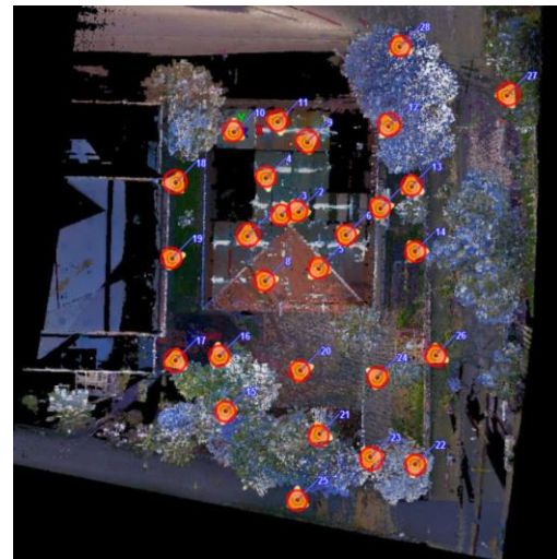
Fig. 2. Top view of area showing laser scanner set-ups
