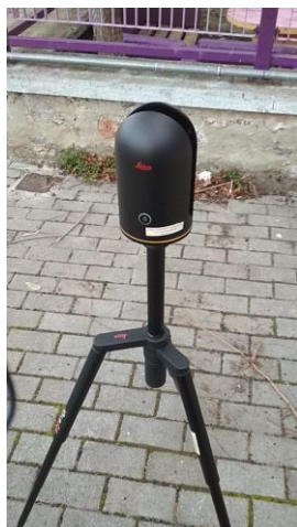
Fig. 1. The BLK360 laser scanner during data collection
