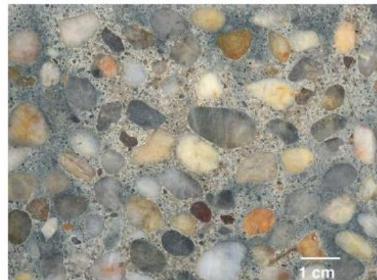
Figure 3. Cross-section of concrete with 6.35-12.7 mm natural aggregates
