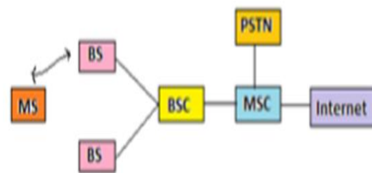
Figure 2. Architecture of Advance Mobile Phone Services (AMPS)
