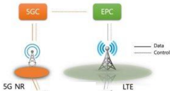
Figure 9. High-level 5GC SA Option 2 interworks with EPC
