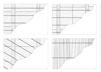
Figure 5. Squemes showing variations in tabique and quincha infills. a. 'Tabique' with single horizontal adobe and horizontal wiring b. 'Tabique' with double vertical adobes and horizontal wiring c. 'Tabique' with single horizontal adobe and diagonal wiring d. 'Quincha' with vertical tobacco branches confined with horizontal wiring.
