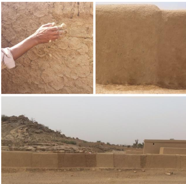
Figure 10. Plaster tests on a new mudbrick structure, from top left: Sample A, coat 1 ; Sample 1, coat 2 ; Samples on the west side of the wall.
