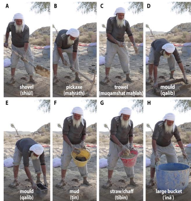
Figure 5. The different tools used throughout the mudbrick production process and their transliterated (local) Arab name.
