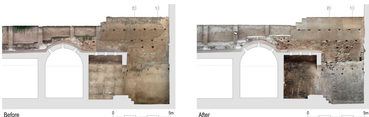
Figure 2. Elevation of the west dividing wall of the Bañuelo. State before and after the consolidation works (section pl. 1-2 marked).
