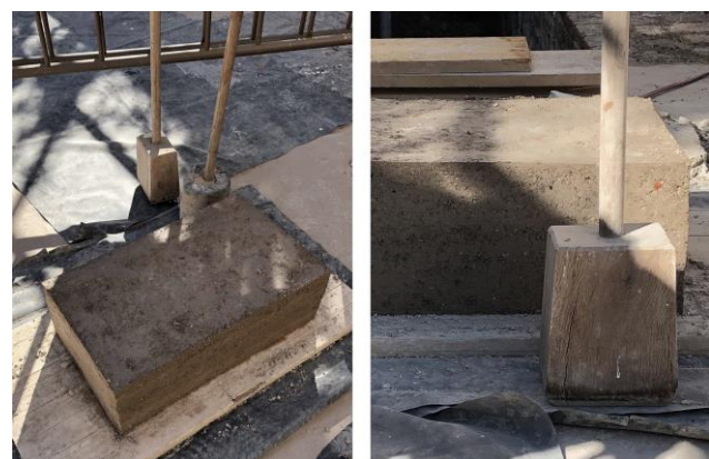
Figure 5. Rammed earth test specimen built in-situ .
