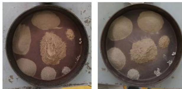
Figure 8. Breakdown and grain size of the adobe samples. Photo: David Preciado Villicaña (2019). © SPOT Image Copyright 2020.
