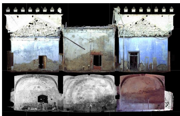
Figure 10. Ortho-image from laser scanning data from which drawings can be obtained.
