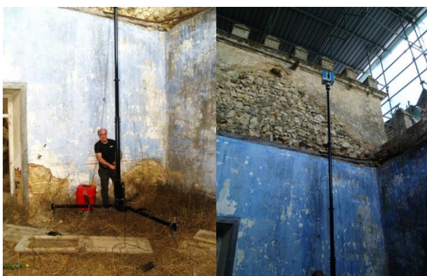
Figure 7. Using a hydraulic mast to reach the higher parts of the building.
