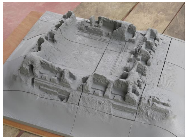
Figure 12. Final 3D printed model of the Acropolis consisting of 17 parts reassembled in La Blanca.
