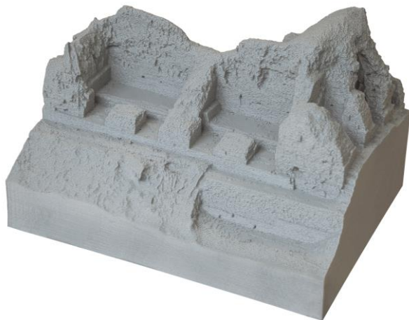
Figure 10. Print tests in scale 1:100 and accuracy 0.3 mm.
