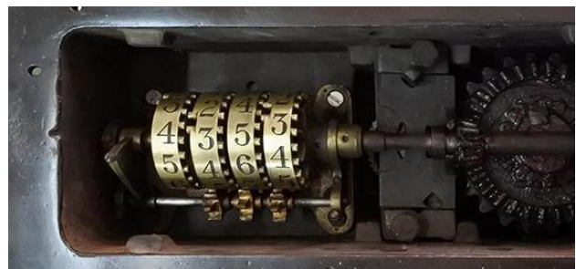
Figure 11. Cordillera elevator turnstile counter.
