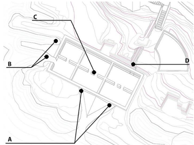
Figure 2. Fish farm type model, using the example of Baños de la Reina in Calp (Alicante): (A) Water supply channels, in the direction of the sea waves; (B) Water outlet channels; (C) Fish tank with internal subdivision; (D) Possible sweet water supply channel.
