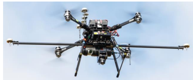
Figure 2. Vulcan Raven aircraft carrying Routescene UAV LiDAR System LidarPod and GNSS antennas, and Sony α6000 payloads.
