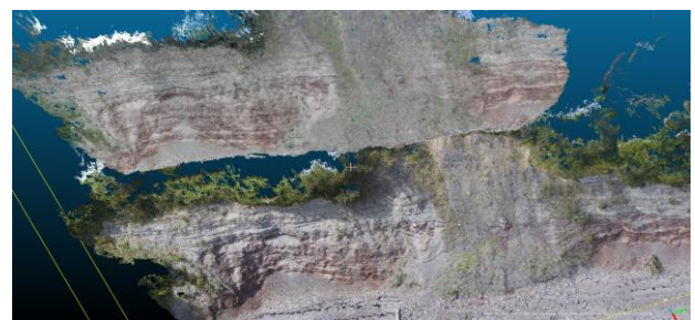
Figure 18. Like-to-like Alignment (Pole Survey up and Drone Survey down)
