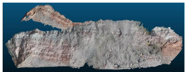
Figure 8. Multiple Block Point Cloud Showing the Effect of Drifting on the Inexpensive GNSS Sensors
