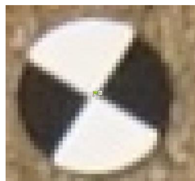
Figure 2. Ground control target as it appears in photograph.
