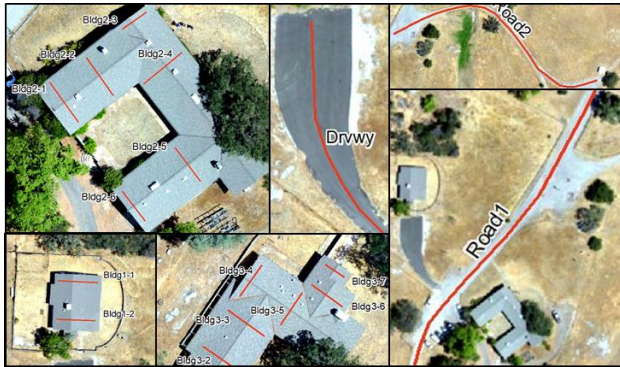
Figure 3. Features and profile paths for elevation profile analysis.
