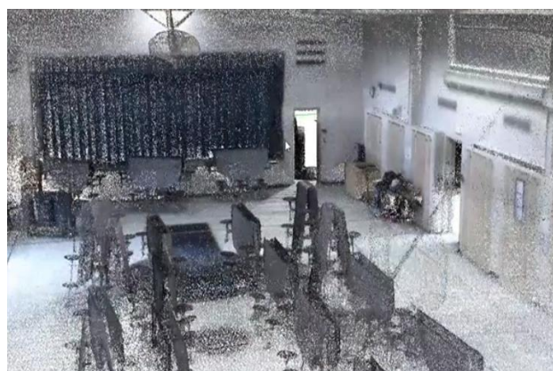
Figure 1: Spherical imagery (top) and colorized point cloud (bottom) viewed in Paracosc's Retrace and Rapidlasso's LasTools software, respectively.
