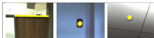
Figure 3: Representation of example feature types as lines or points (yellow) in Retrace including door (left), fire alarm (middle), and smoke detector (right).
