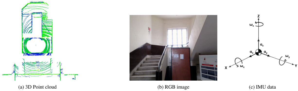
Figure 3. Data captured from the proposed system (a): point cloud data (top view), (b): RGB image, and (c): IMU data (accelerometer and gyroscope data)
