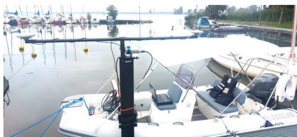
Figure 3. RIB boat with integrated Norbit Portus measurement system
