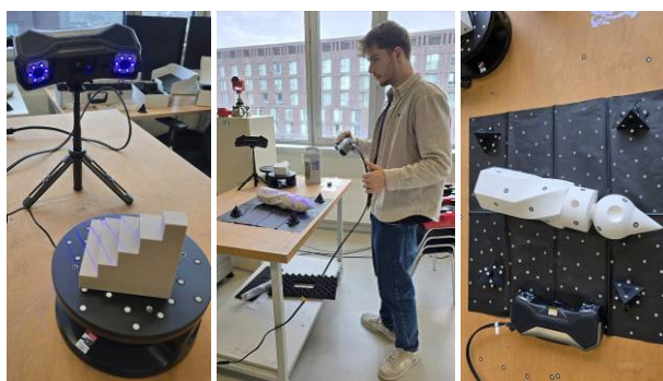
Figure 3. Scanning of the stairways on the turntable with MetroX (left) and scanning of the Testy on a black plastic mat with targets.
