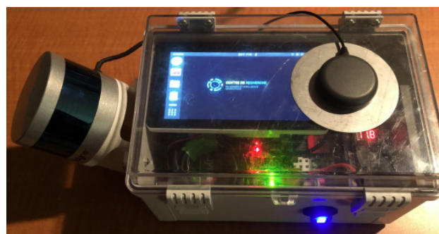
Figure 8. In-house mobile scanning system which integrates a VLP-16 LiDAR scanner and VN200 GNSS/IMU unit.
