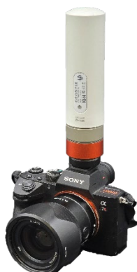
Figure 1. GEOSTIX-X5 GNSS receiver attached to Sony A7R III camera via the flash sync port (hot shoe).
