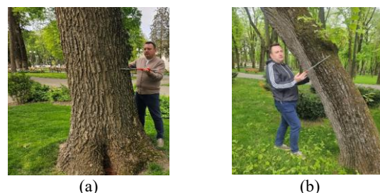
Figure 5: Measuring DBH in the field using a forest caliper: straight trunk (a) and inclined trunk (b)
