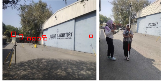
Figure 3. Experiment setup in outdoor environment. Ground truth is estimated by total station survey.
