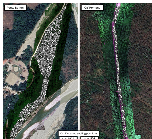
Figure 2. ULS-derived sapling detections along the two study areas. White points indicate the positions of detected saplings; totals are n = 5427 at Ponte Baffoni and n = 801 at Ca' Romano.
