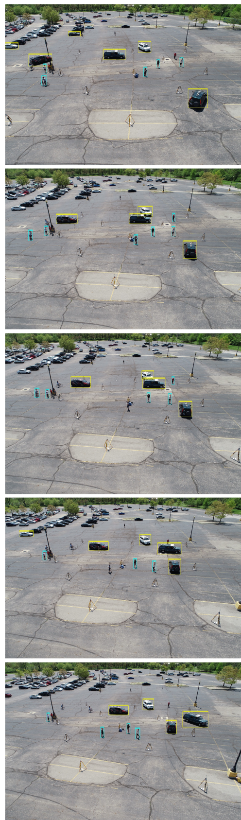
Figure 3. Sequence of UAV camera views: detected ground vehicles are shown with yellow boxes, whereas light blue boxes indicate the detected pedestrians.
