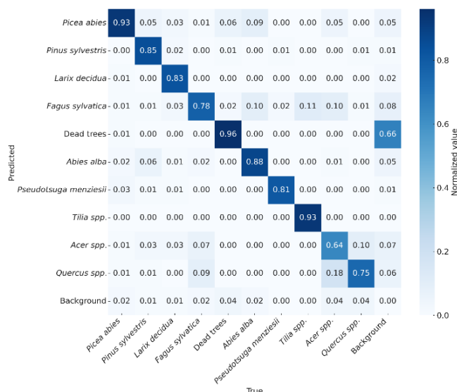
Figure 5. Normalized confusion matrix of the YOLO11x model trained on the balanced masked dataset after hyperparameter tuning (173 epochs).
