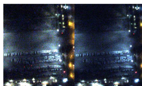
Figure 3. CO3D demosaiced night image of Istanbul acquired with a 70ms integration time, before (left) and after (right) defective pixels interpolation.
