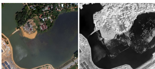
Figure 10: Example of 50 cm resolution RGB and NIR images over Vietnam – © CNES-Airbus
