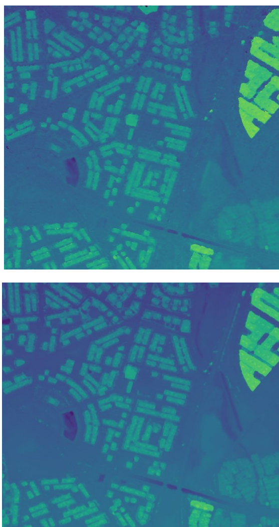
Figure 17: Comparison of 2 extracts of DSM of Marrakech. Top: CO3D, Bottom: Pleiades-Neo reference.
