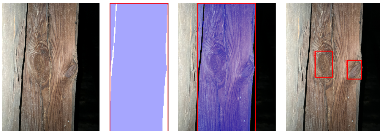
Figure 2. AI-pipeline for wood knot detection: RGB image (a), segmented beam side boundaries mask (b) applied on RGB image (c) and detected wood knots inside segmented boundaries (d).
