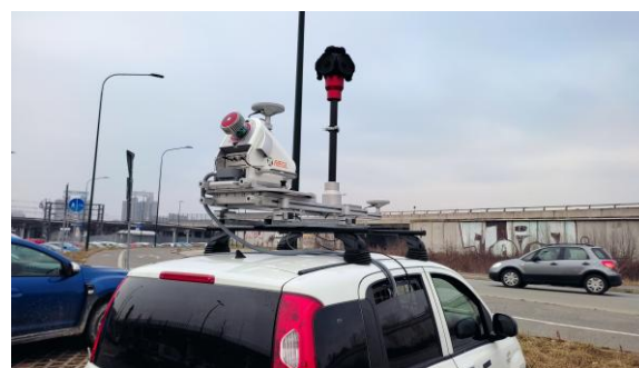
Figure 3. The MMS RIEGL VMX-2 mounted on the vehicle for ground-based acquisition.
