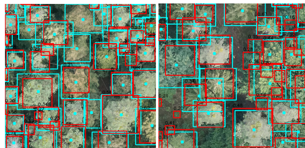
Figure 2. Types of prompts used - point prompts and bounding box prompts (in cyan) derived from ground truth labels, and automatic bounding box derived using DeepForest method (in red)
