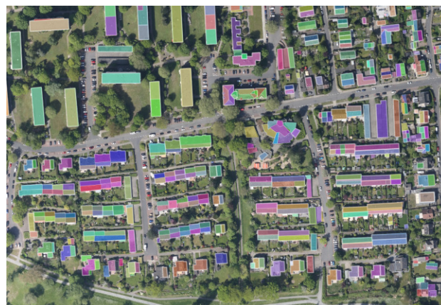
Figure 7. Graph-based 2D roof planes vectorization.
