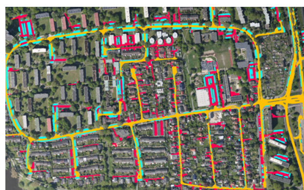
Figure 5. Example of traffic areas segmentation results in Schwarzer Berg. Class colors are: ■ parking area, ■ road, ■ access way.
