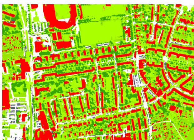
Figure 4. Example of semantic segmentation results in Schwarzer Berg. Class colors are: ■ impervious surfaces, ■ buildings, ■ low vegetation, ■ trees, ■ cars.
