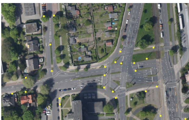
Figure 9. Detected poles, highlighted with yellow dots.
