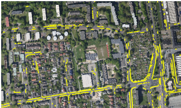
Figure 8. Extracted curbstone lines.
