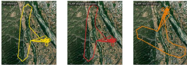
Figure 5. Planimetric comparison of the AT reference trajectory, the proposed aligned SLAM trajectory, and the S+T baseline.
